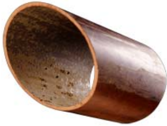
ABOVE: Interior view of pitting, which leads to pinhole leaks in a copper pipe.
