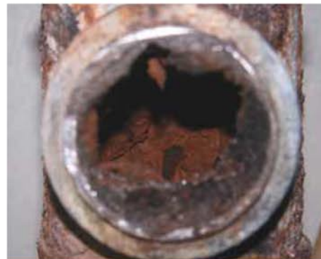
Tuberculation or build-up of scale inside a galvanized pipe reduces internal pipe diameter, consequently affecting water flow and water pressure
